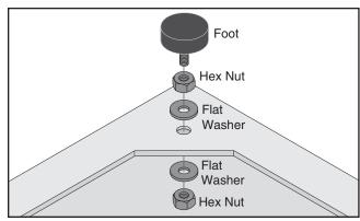
Figure 10. Stand foot installed (1 of 4).
